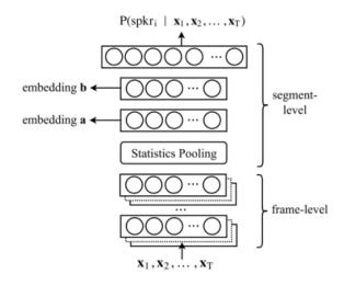
The first five layers of time-delay network are frame-level, The sixth layer is a statistics pooling layer, which is responsible for calculate the mean and standard deviation of frame-level and map it to segment-level layer. After getting the embedding, also use PLDA to do speaker classification. If there are sufficient data, X-vector can get better performance. Table 1 is the detail of input dimension and context of every level.
